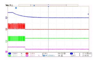
Note: (1)Channel(BLUE) is VEN, Channel2(RED) is I of Inductor, Channel3(GREEN) is VSW, Channel4(PINK) is VLED+ (2)For guaranteed effects the DIMMING frequency is suggested within 2KHz.
